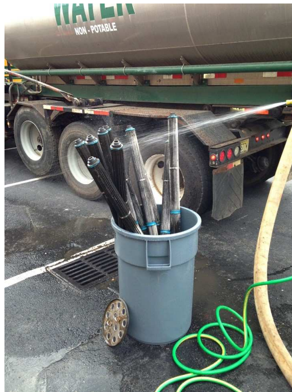
Rinsing of dirty filter cartridge tentacles with a low-pressure garden hose sprayer, and using a plastic garbage container to capture rinse water.
